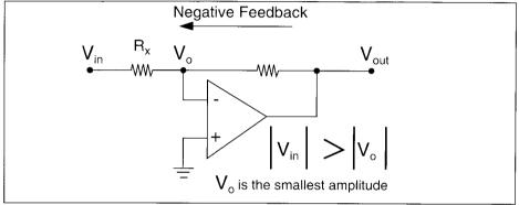
Figure 1. Amplifier with negative feedback.
