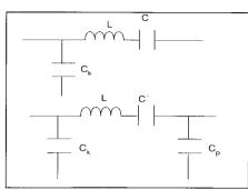
Figure 8. End section (top) and matched end section (bottom)
