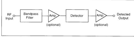
Figure 2. The TRF receiver includes a filter before signal detection, and may also include RF amplification, baseband amplification and other signal processing.
