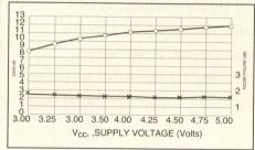
Figure 6. Gain and NF vs supply voltage.
