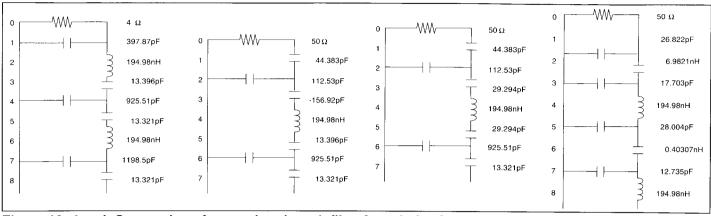
Figure 10a,b,c,d. Conversion of narrowband mesh filter from 4 ohm impedance to 50.
