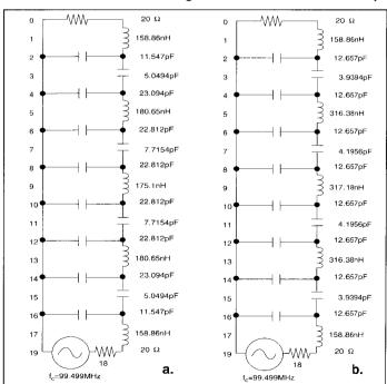
Figure 2a. Initial sytnthesis of bandpass filter. Figure 2b. Filter after equal-value transformation.
