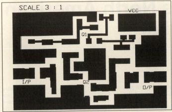
Figure 4. Printed circuit board for LNA without component locations.
