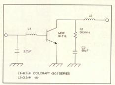
Figure 2. LNA schematic.
