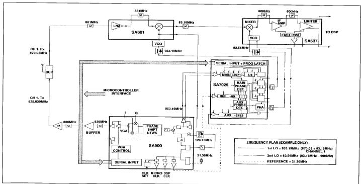
Figure. 1 Block diagram of TDMA IS-54 chip set.
