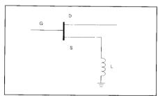
Figure 1. The inductor between the source lead and ground insures stabilitity.
