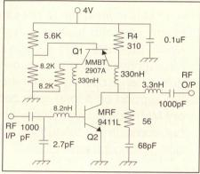
Figure 3. LNA schematic including DC bias.
