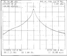
Figure 9. Frequency response of the RF receiver.
