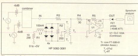
Figure 5. Schematic of final AGC and test set-up
