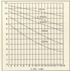
Figure 3. Noise resistance versus feedback inductance.
