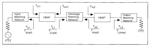
Figure 10. Admittances for two-stage amplifier.
