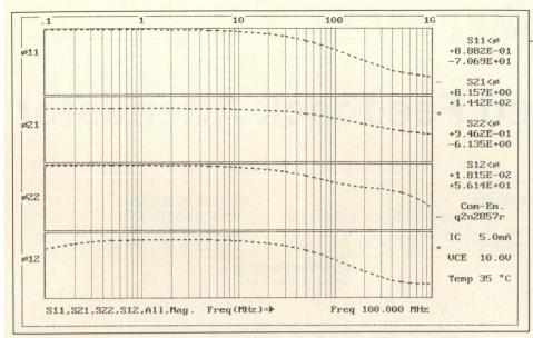
Figure 4. S-Parameter magnitude plots for the 100 MHz amplifier.
