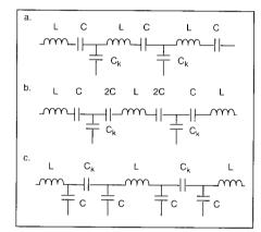
Figure 1. Transformation of a filter to the tubular form.
