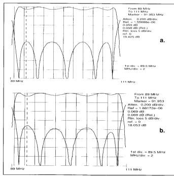
Figure 3a. Calculated response of original filter. Figure 3b. Calculated response of transformed filter.
