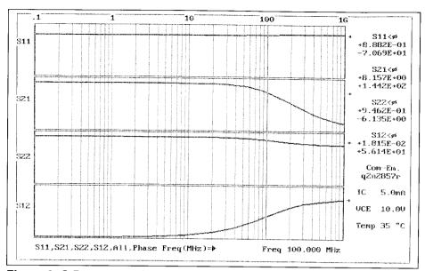
Figure 3. S-Parameter phase plots for the 100 MHz amplifier.
