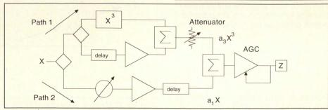
Figure 4. Block diagram of the pre-distorter.
