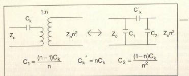
Figure 4. Norton's first transformation applied to a capacitor.
