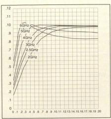
Figure 2. Variation of stability factor (K) versus inductance.
