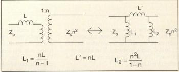
Figure 6. Norton's first transformation applied to an inductor
