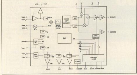
Figure 5. Block diagram of SA900.
