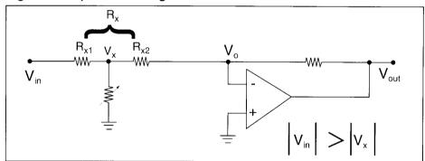
Figure 2. Attenuator placed at a point between V<sub>in</sub> and V<sub>out</sub>
