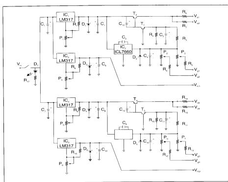
Figure 8. Circuit diagram of the Built In Test Equipment.
