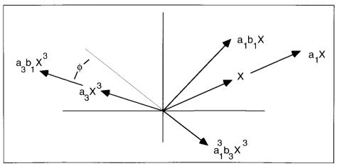
Figure 2. Vector representation of input signal, pre-distortion signal, and signals after amplification.
