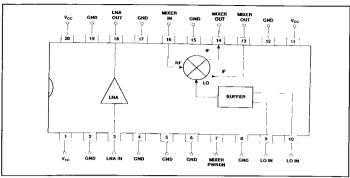
Figure 2. Block diagram of SA601.
