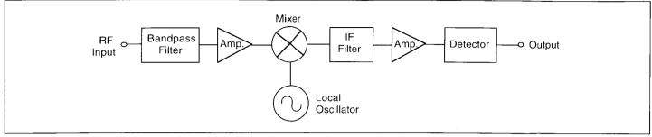
Figure 4. The single-conversion superhetrodyne receiver can be described as a frequency conversion stage preceding a TRF or direct-conversion receiver. Other detector options include FM, I and Q, or logarithmic.
