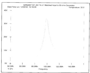
Figure 2. Narrowband gain plot of the amplifier.
