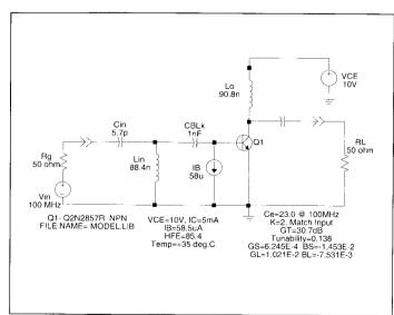
Figure 1. 100 MHz tuned amplifier circuit.
