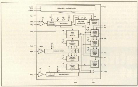
Figure 4. Block diagram of SA7025.
