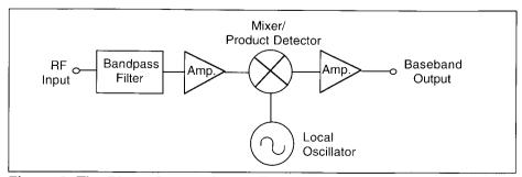
Figure 3. The Direct-Conversion or Zero-IF receiver performs frequency translation from RF to baseband.
