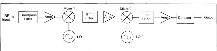
Figure 5. The double-conversion superhetrodyne architecture adds another frequency conversion stage, usually to aid in rejection of image signals. Triple and quadruple conversion schemes may also be used.
