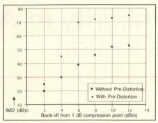
Figure 3. IMD vs. input power pullback from 1 dB compression point with pre-distortion and without.
