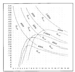
Figure 7. Variation of  $G_{T(opt)}$  and  $G_{T(max)}$  with frequency.
