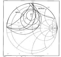
Figure 1. Gain and NF contours for MRF9411L.
