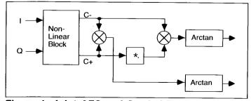
Figure 1. Joint AFC and Symbol Timing Recovery Algorithm
