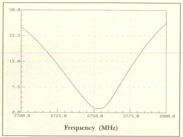
Figure 10. Noise figure of the RF receiver.
