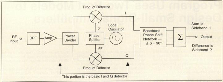
Figure 5. A complete I and Q based receiver, using the phasing method of SSB demodulation. The I and Q detector portion of the circuit is noted.
