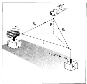
Figure 1. Geometry for the bistatic radar.
