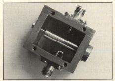
Figure 4. Bandpass RF filter.
