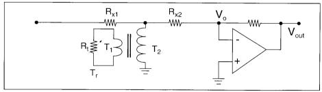
Figure 3. Transformer T, reduces the voltage across R,
