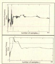
Figure 8. The estimated response in the presence of delay dispersion
