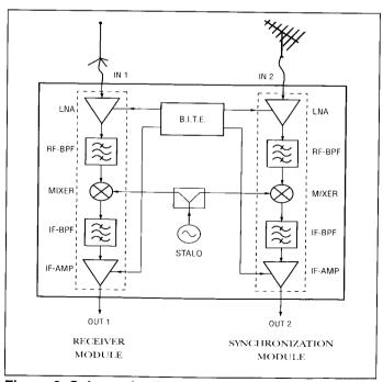
Figure 2. Schematic diagram of the RF receiver.
